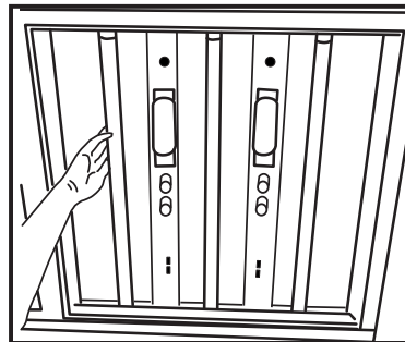
2. Remove the fluorescent Tubes & ballast
